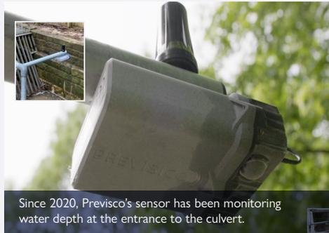
Since 2020, Previsico's sensor has been monitoring water depth at the entrance to the culvert.
