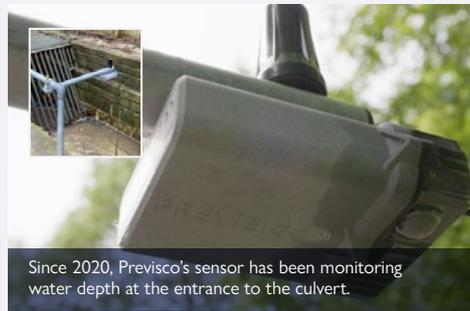
Since 2020, Previsico's sensor has been monitoring water depth at the entrance to the culvert.
